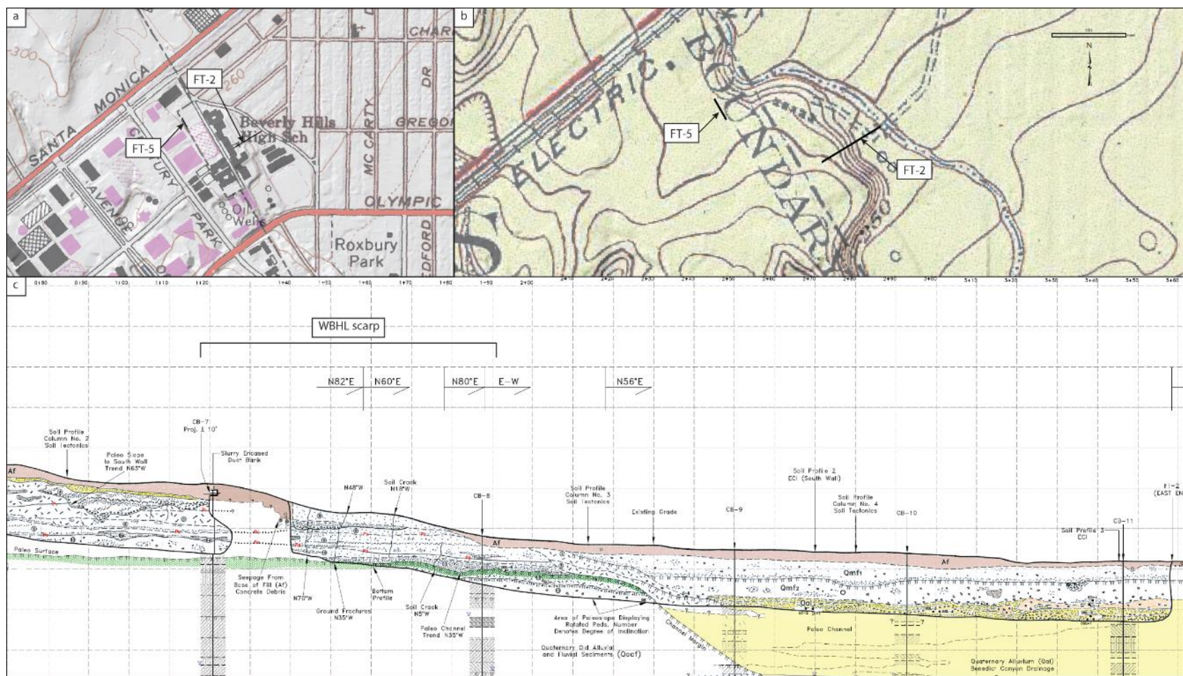
Figure 17 - a) Index map showing location of trenches FT-2 and FT-5 on modern topographic base map. b) Trench locations on 1925-era topographic map showing WBHL scarp prior to modification. c) Portion of geologic cross section and fault trench log for FT-2 at Beverly Hills High School (from Leighton Consulting, Inc., 2012a, Plate 3). Af = artificial fill; Qmf = mud flow deposits (Holocene); Qal = alluvium (Holocene); Qoaf = older alluvial fan deposits (late Pleistocene)
