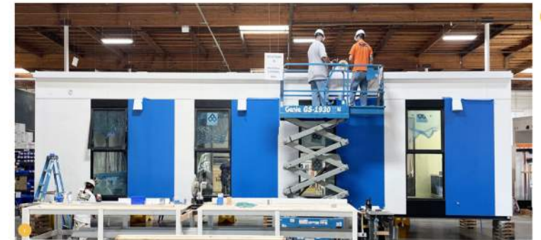
STATION 09: CS-05A: Gutters and interior finishes are being installed at station 9.
